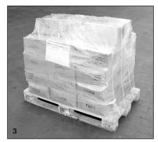
3 - Accessories such as joint components, screws, nuts, dowels etc, are packed within cardboard parcels. in order to prevent screws, nuts, washers and dowels from rusting., they firstly are put into nylon bags. All parcels are prepared not exceeding 25kg and are identified by labels indicating product information. Small product packages then are stacked onto wooden palette and wrapped against scattering and supported on the sides using PVC strapping.
